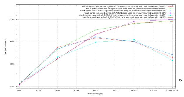
and the second type, where random writes with small and large IO block size are fast, but with medium IO block size are slow:
