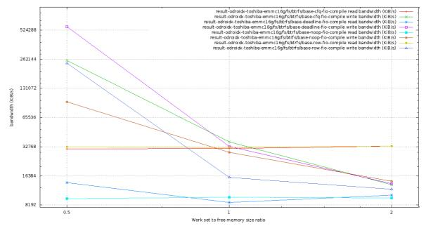
Write performance starts with very high numbers when work set is small and drops to nearly direct linear medium write speed at big work set size. Read performance varies insignificantly with work set size change, but highly depends on selected IO scheduler and a little less on file system options. Noop scheduler shows the worst aggregated throughput, CFQ and ROW show the best. Both read and write throughput variation with file system options and IO scheduler selection reaches 400%:
