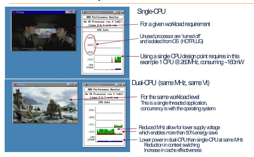
Once you have threaded code, MP offers more performance at lower MHz and without suffering from the cost of memory speed disparity and associated inefficiencies
