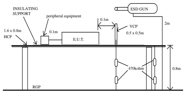
The reference ground plane size projects beyond the horizontal coupling plane by at least 0.5 m on all sides.
