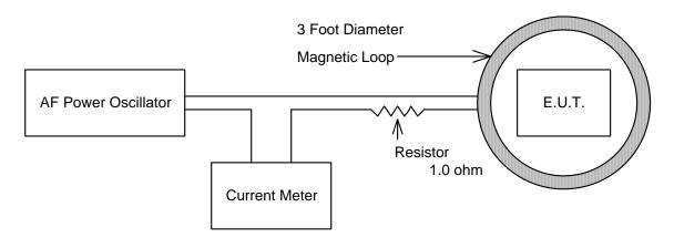
The current meter is used to calibrate the magnetic field
