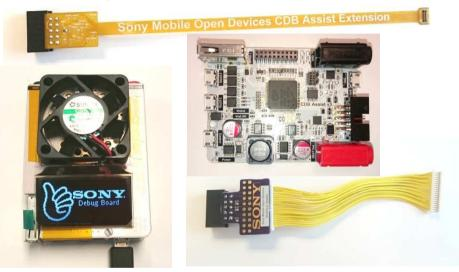
Adapters to connect directly to internal debug port in Xperia devices and to development boards.
