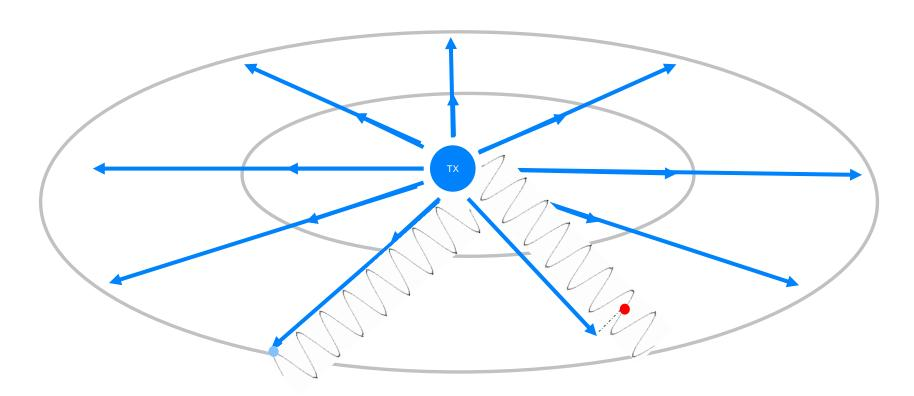
But with 2 antennae at different distances from the transmitter
