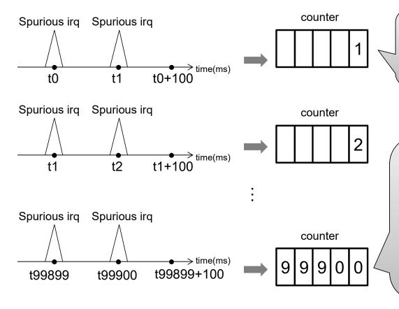
• Increment counter if spurious interrupt occur within 100ms of the previous spurious interrupt.
