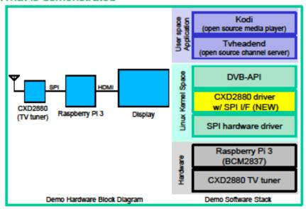
The CXD2880 receives DVB-T2/T signals and transfers an MPEG-2 transport stream via a SPI bus to the Raspberry Pi for picture decoding. An embedded MPEG-2 TS Packet ID (PID) filter reduces the data rate, which makes streaming over SPI possible. The CXD2880 driver is running in the Linux kernel space and has the common DVB API.
