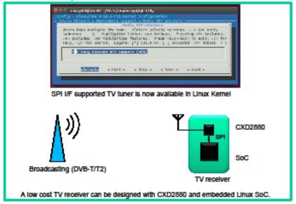
Single board computers have become popular. A low power TV tuner CXD2880 features SPI interface allowing direct attachment to a single board computer such as Raspberry Pi to make your own TV receiver with open source software. It may also be extended to new broadcasting services.
