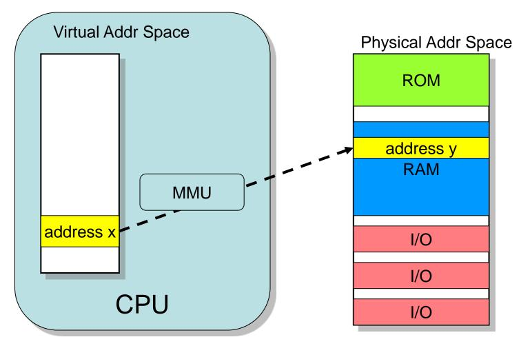
Only physical addresses come out of CPU onto address bus. Virtual addresses can not be observed with the logic analyzer
